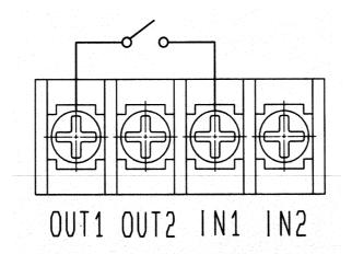
Fig. 21. Wiring for temporary stop
