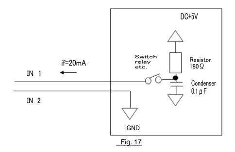
Temporarily stop operation: Switch / relay contact OFF Re-Start Operation: Switch / relay contact ON
