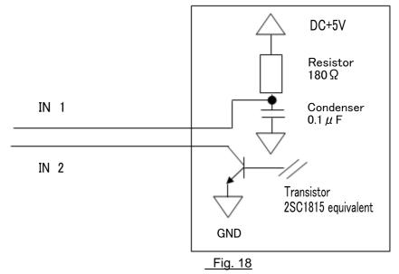
Temporarily stop operation : Transistor OFF Re-Start Operation: Transistor ON
