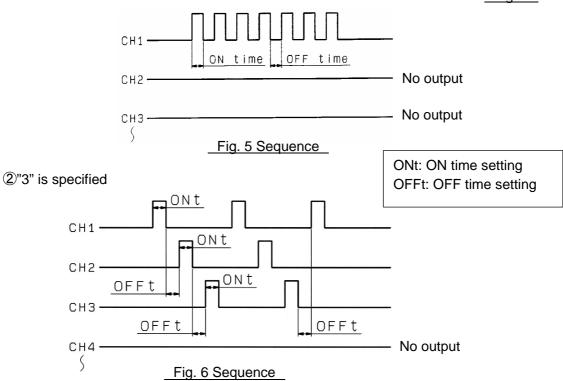
2) Setting the number of energizations (1 or 2). Determine which valves to have 1 or 2 outputs, and set the dip switch for the correct setting. (ON: twice, OFF side: once)
