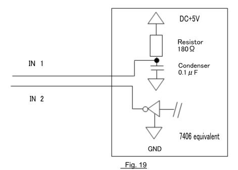
Temporarily stop operation: Open collector OFF Re-Start Operation: Open collector ON
