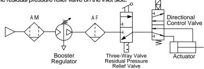
• Release the supply pressure with the residual pressure relief valve after operation is stopped. Stop unnecessary motion of the booster regulator to prevent switching failure that occurs below the minimum operating pressure or less.
