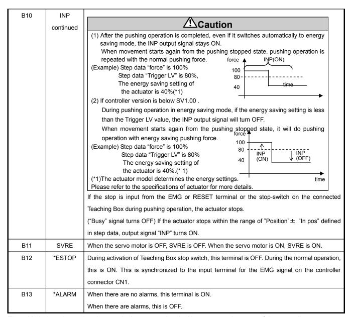
The table below shows the changes in the output signal with respect to the state of the controller.
