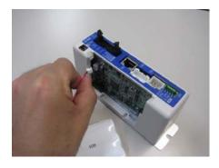
4) When installing the battery case, ensure that the cable is not trapped between the battery case and the controller housing .
