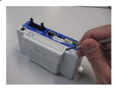
4) Detach the battery connector from the controller PCB.
