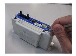
2) Disconnect the battery connector from the circuit board.
