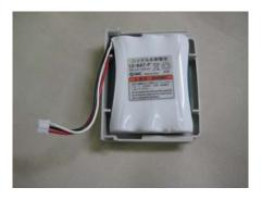
3) Connect the replacement battery to the circuit board.
