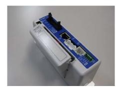
8) Carefully push the battery case into the controller housing until fully installed. Confirm that the battery case does not move.
