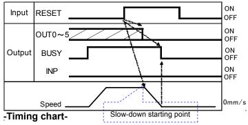
\* If the actuator is within the "In position" range, INP will be turned ON.
