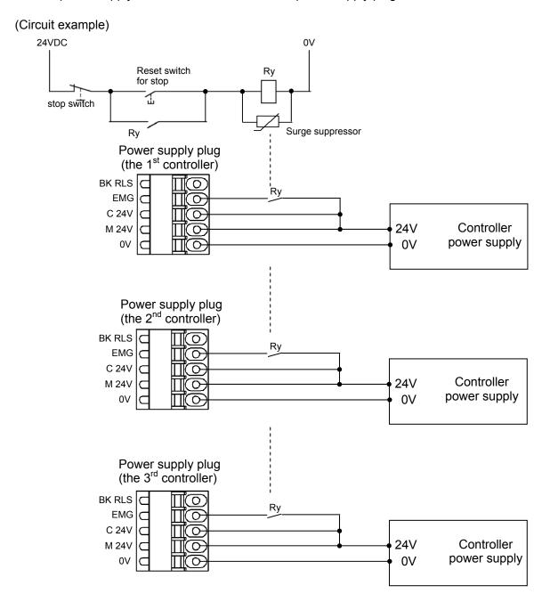
The relay must be a safety relay or monitored by a safety relay.
