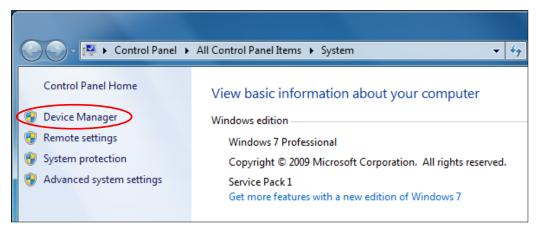
iv. Double-click "Other Devices", select the "SMC Serial Converter" with the "!" symbol and right-click to open the menu shown below on the left. Select "Update Driver Software".
