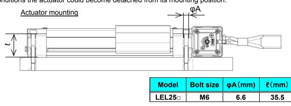
4. When mounting the actuator, leave a gap of 40mm or more to allow for bending of the actuator cable.
