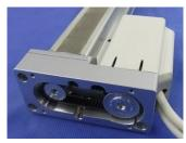
2."Motor cover" and "Grommet" are removed. (Only "With motor cover")
