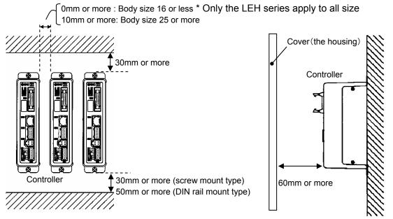
Install the controller on a flat surface. Excessive pressure applied to the housing will damage the controller.
