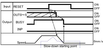
\* If the actuator is within the "In position" range, INP will be turned ON.
