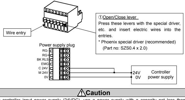
For controller input power supply (24VDC), use a power supply with a capacity not less than the "momentary maximum power" of the actuator specifications. Do not use "inrush-current restraining type" power supply.
