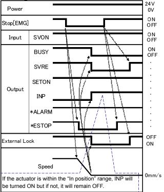
\* The "ALARM" and "ESTOP" are expressed as negative-logic circuit. \* When "Stop" is OFF, the stop is activated.
