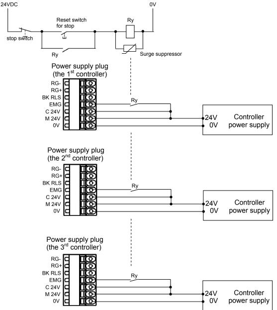
(Circuit example) \* The figure below shows the stopped state.
