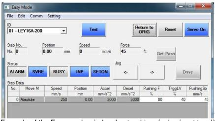
Example of the Easy mode window (motor driver (pulse input type))
