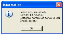
When the test mode is switched to the monitor mode, the following notice is shown. Note that the controller parallel IO becomes valid.
