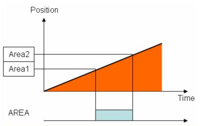
The AREA output is a signal to be output when the position enters the specified range. The AREA 1 and AREA 2 in the setting items define this output range.
