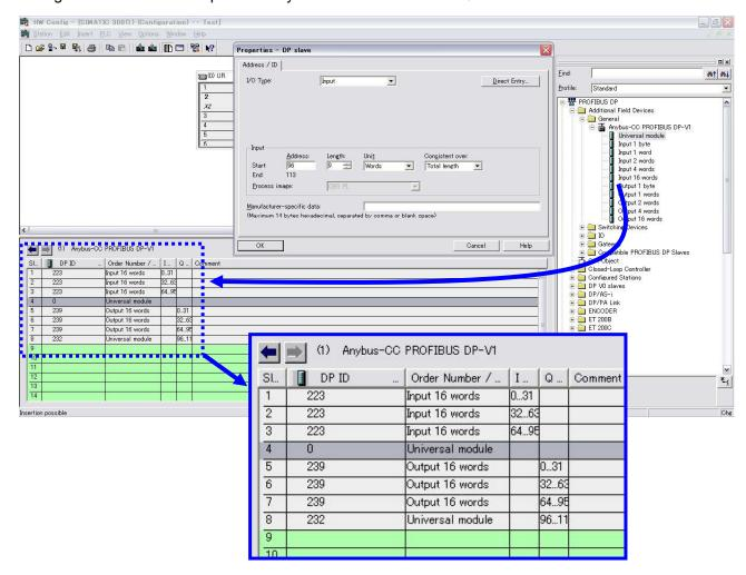
It is set completion by downloading the configuration data to PLC.
