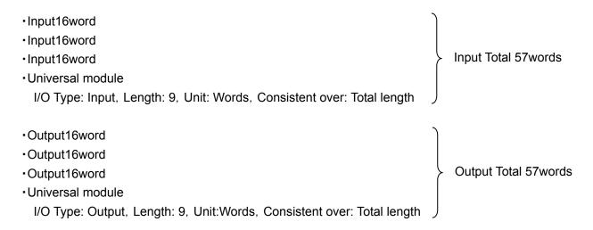
Please give "I Address" and "Q Address" to me with the crack so as not to overlap. The figure below is an example to set by "I Address 0-113" and "Q Address 0-113".
