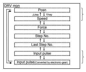
TB Ver2.1\* or more: When connecting to LECPA, "Position" and "Speed" is displayed by the unit of "mm(or degree)" and "pulse".
