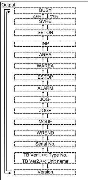
\*Parallel I/O only in connecting controller can be monitored. In Output signal monitor items, the signal that is not in connecting controller is displayed but cannot be monitored.
