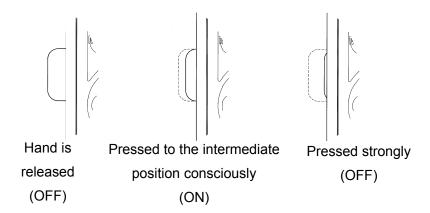
During the manual operation, if an unexpected actuator motion occurs, releasing or strongly pressing enable switch on the teaching box stops the actuator motion and the motor power turns off (servo OFF)
