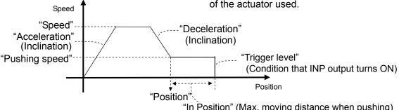
"In Position" (Max. moving distance when pushing)
