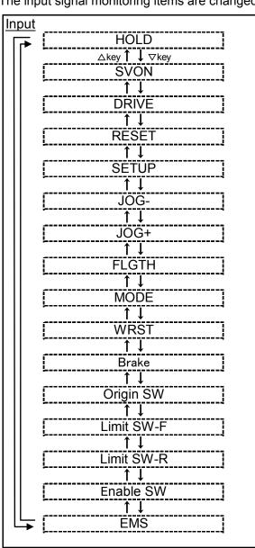
\*Parallel I/O only in connecting controller can be monitored. In lutput signal monitor items, the signal that is not in connecting controller is displayed but cannot be monitored.
