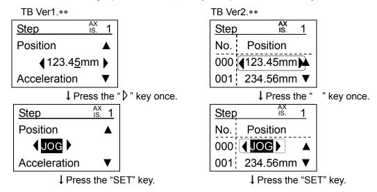
② EXT Inp OFF: To confirm whether to disable the input from external equipment such as PLC. It is necessary to be disable the input from outside to do "JOG input" operation.
