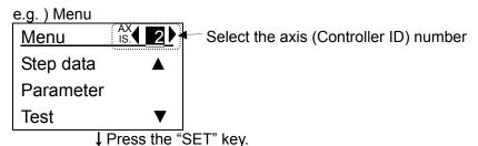
After that, it is possible to execute the setting, test, monitor and file for the selected axis (controller).
