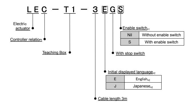
\*1 When a teaching box with enable switch is selected, it is necessary to activate the enable switch to change the default parameter setting of the controller.
