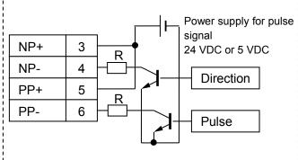
NPN open collector input for 1 pulse mode \*1)
