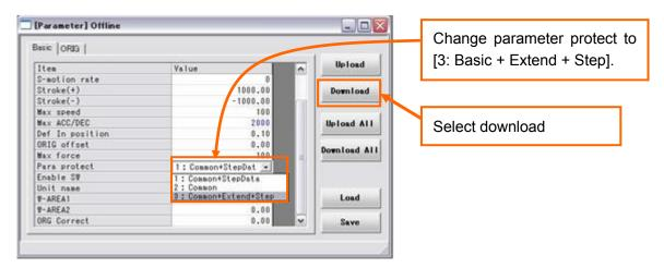
Change the parameter window "Basic"-"Parameter protect" to "3: Basic + Extension + Step" Select "Download" button. The modified data is transmitted to the driver. Once downloaded, the parameter set value which was displayed in blue will now be displayed in black.
