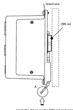
Hook the driver on the DIN rail and press the lever of section A in the arrow direction to lock it.
