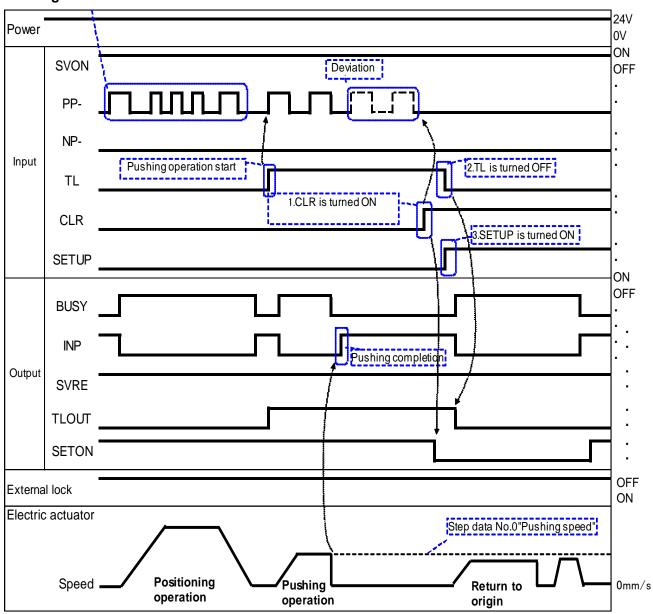
Example2) Not clear the deviation. Input the pulse for the distance of pushed electric actuator but in the opposite direction with TL input ON.
