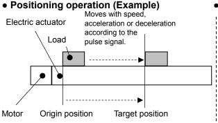
Positioning operation [Speed/ Position] (Example)
