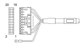
Connected to the cable shield Be sure to provide grounding.
