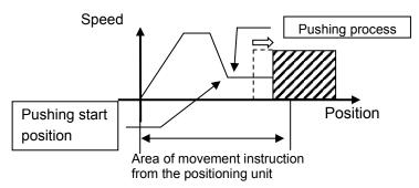
(ii)When the electric actuator moves in the opposite direction of pushing direction
