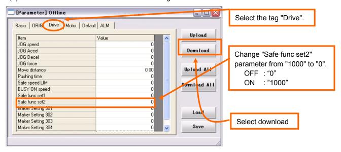
Select the "Download" button. The modified data is transmitted to the driver. Once downloaded, the parameter set value for "Safe func set2" which was displayed in blue will now be displayed in black.
