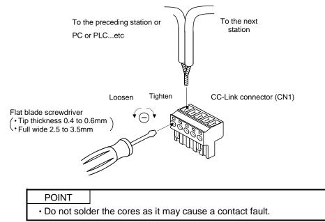
Use of a flat-blade torque screwdriver is recommended to manage the screw tightening torque. The following table indicates the recommended products of the torque screwdriver for tightening torque management and the flat-blade bit for torque screwdriver. When managing torque with a Phillips bit, please consult us.
