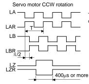
Time cycle (T) is determined by the settings of parameter No.PA15 and PC19.
