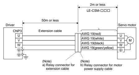
Note. Use of the following connectors is recommended when ingress protection (IP65) is necessary.
