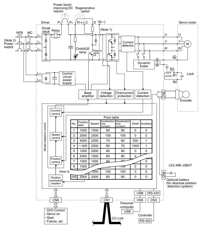
Note 1. The built-in regenerative resistor is not provided for the LECSC $\Box$ -S5.
