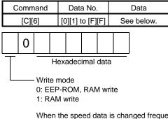
When the speed data is changed frequently through communication, set "1" to the write mode to change only the RAM data in the driver. When changing data frequently (once or more within one hour), do not write it to the EEP-ROM.
