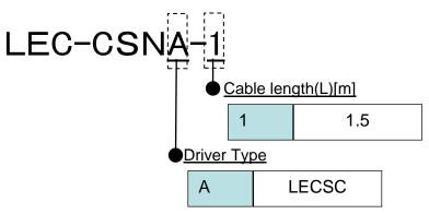
\*LEC-CSNA-1 is 10126-3000PE(Connector)/10326-52F0-008(Shell kit) of Sumitomo 3M Limited or equivalent goods.
