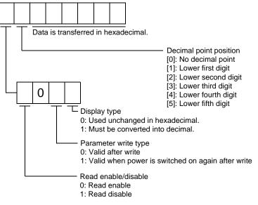
For example, data "1200270F" means 999.9 (decimal display format) and data "0003ABC" means 3ABC (hexadecimal display format).
