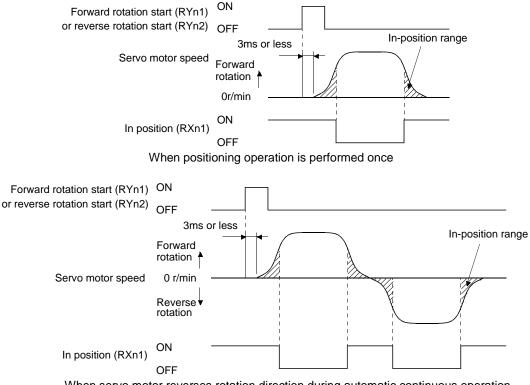
When servo motor reverses rotation direction during automatic continuous operation
