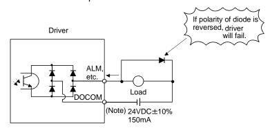
Note. If the voltage drop (maximum of 2.6V) interferes with the relay operation, apply high voltage (up to 26.4V) from external source.
