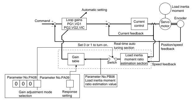
When a servo motor is accelerated/decelerated, the load inertia moment ratio estimation section always estimates the load inertia moment ratio from the current and speed of the servo motor. The results of estimation are written to parameter No.PB06 (the ratio of load inertia moment to servo motor). These results can be confirmed on the status display screen of the set up software (MR Configurator2<sup>™</sup>) section.
