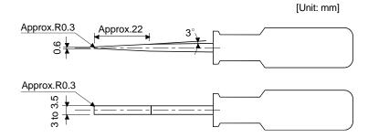
2) When using the flat-blade screwdriver - part 1
