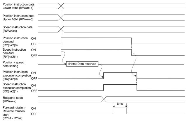
Note. This data is stored into RAM of the driver. Hence, the data is cleared when power is switched off.
