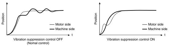
When the advanced vibration suppression control (vibration suppression control tuning mode parameter No.PB02) is executed, the vibration frequency at machine side can automatically be estimated to suppress machine side vibration.
