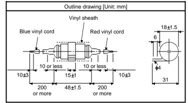
Note that a diode should be installed to a DC relay, DC valve or the like.
