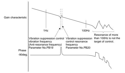
(b) When vibration can be confirmed using monitor signal or external sensor
