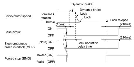
Note. ON: Lock is not activated. OFF: Lock is activated.
