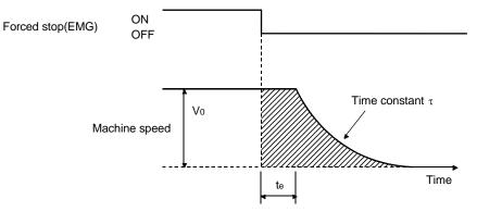
Fig. 12.3 Dynamic brake operation diagram
