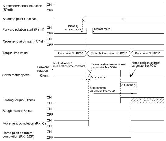
Note 1. Configure a sequence that changes the point table selection earlier, considering the delay time of CC-Link communication.
