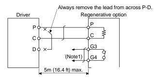
Note 1. Make up a sequence which will switch off the magnetic contactor (MC) when abnormal heating occurs.
