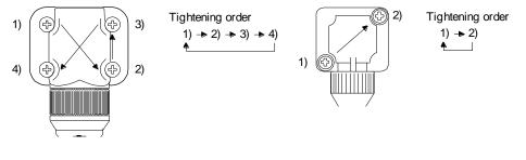
Connector for power supply, connector for encoder
