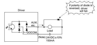
Note. If the voltage drop (maximum of 2.6V) interferes with the relay operation, apply high voltage (up to 26.4V) from external source.
