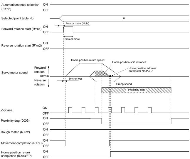
Note. Configure a sequence that changes the point table selection earlier, considering the delay time of CC-Link communication.
