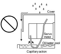
(2) If oil such as cutting oil drops on the servo motor, the sealant, packing, cable and others may be affected depending on the oil type.
