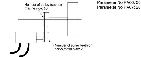
(b) Example 2 When the number of pulley teeth on the machine-side is 50, the number of pulley teeth on the servo motor side is 20, and using the servo motor with 1/9 reduction gear.
