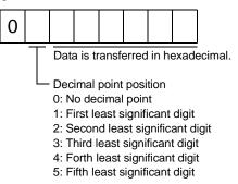
By way of example, here is described how to process the set data when a value of "15.5" is sent. Since the decimal point position is the second digit, the decimal point position data is "2". As the data to be sent is hexadecimal, the decimal data is converted into hexadecimal.  $155\rightarrow 9B$
