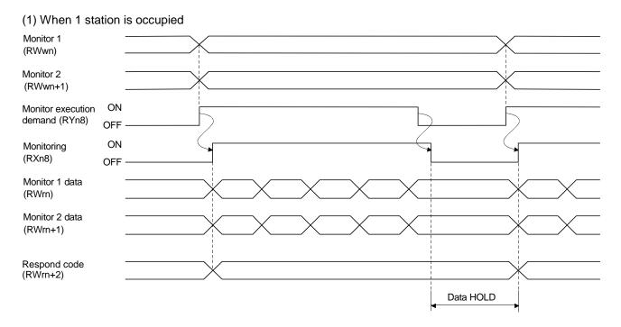
Set the monitor codes No. (0000 to 001D) (refer to section 3.5.3) to Monitor 1 (RWwn) and Monitor 2 (RWwn+1) and turn Monitor output execution demand (RYn8) to ON. Turning Monitor execution demand (RYn8) to ON sets the next data. Data are all hexadecimal numbers. At this time, Monitoring (RXn8) turns to ON at the same time.
