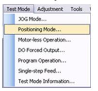
Click " Positioning Mode " on the menu bar and click "Move Distance Unit Selectiom" on the menu. Check Command pulse unit (Electronic gear valid) and click OK. Electronic gear ratio that is set in the PA05 / PA06 / PA07 is enabled.
