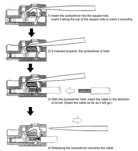
3) When using the flat-blade screwdriver - part 2
