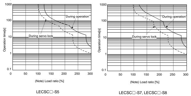
Note. If operation that generates torque more than 100% of the rating is performed with an abnormally high frequency in a servo motor stop status (servo lock status) or in a 30r/min or less low-speed operation status, the driver may fail even when the electronic thermal relay protection is not activated.
