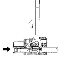
4) Releasing the screwdriver connects the cable.
