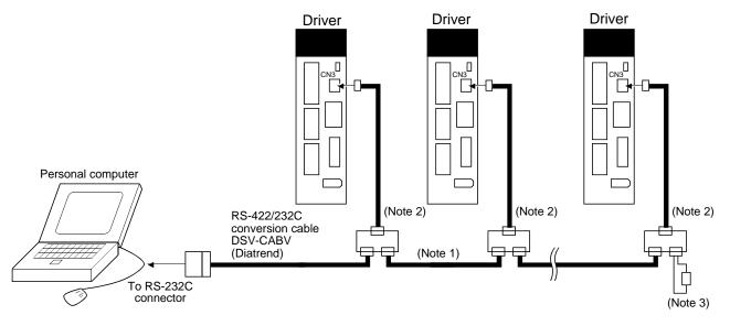
(c) For use of RS-422 to make multidrop connection
