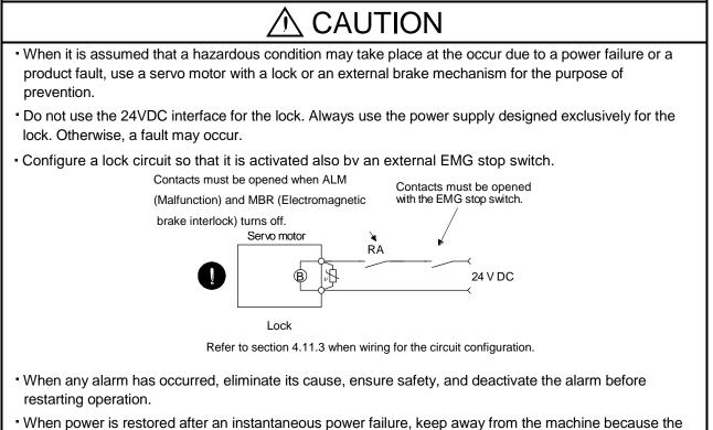
machine may be restarted suddenly (design the machine so that it is secured against hazard if restarted).
