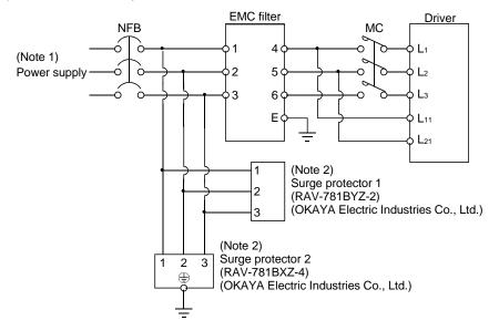
Note 1. For 1-phase 200V to 230VAC power supply, connect the power supply to  $L_1, L_2$  and leave  $L_3$  open.
