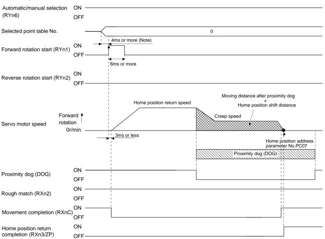
Note. Configure a sequence that changes the point table selection earlier, considering the delay time of CC-Link communication.
