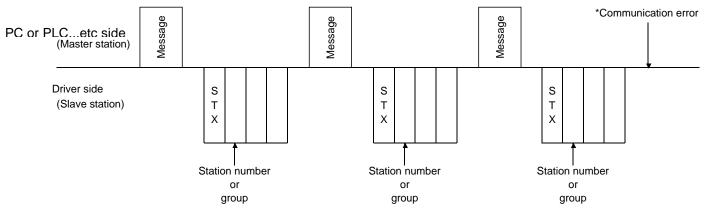
Similarly, when the master station detects a fault (e.g. checksum, parity) in the response data from the slave station, the master station retransmits the message which was sent at the occurrence of the fault. A communication error occurs if the retry operation is performed three times.
