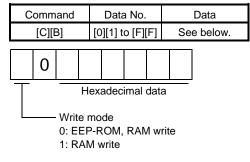
When the auxiliary function constant is changed frequently through communication, set "1" to the write mode to change only the RAM data in the driver. When changing data frequently (once or more within one hour), do not write it to the EEP-ROM.
