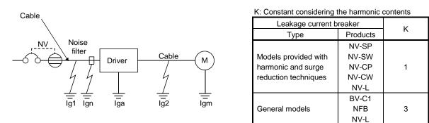
Ig1: Leakage current on the electric channel from the leakage current breaker to the input terminals of the driver (Found from Fig. 13.4.)
