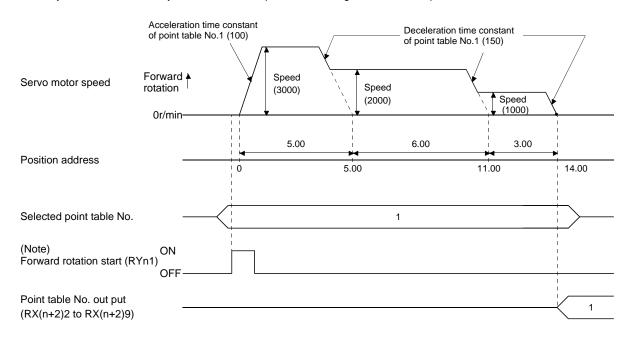
Note. Turning on Reverse rotation start (RYn2) starts positioning in the reverse rotation direction.
