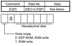
When the acceleration time constant is changed frequently through communication, set "1" to the write mode to change only the RAM data in the driver. When changing data frequently (once or more within one hour), do not write it to the EEP-ROM.
