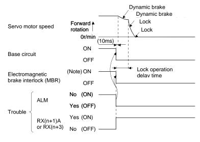
Note. ON: Lock is not activated. OFF: Lock is activated.
