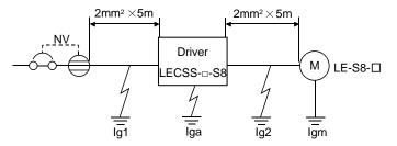
Use a leakage current breaker generally available. Find the terms of Equation (13.1) from the diagram.
