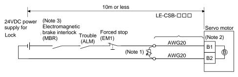
Note 1. Connect a surge absorber as close to the servo motor as possible.
