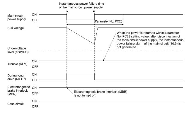
When the instantaneous power failure tough drive function activates, the number of tough drive of the display mode (alarm mode) is increased by one. (Refer to section 5.5.)
