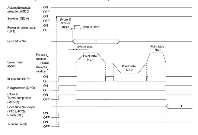
Note 1. External input signal detection delays by the input filter setting time of parameter No. PD19. Additionally, make up a sequence that changes the point table selection ahead of time by considering delays in output signal sequence from the PC or PLC...etc and variations of a signal change due to hardware.
