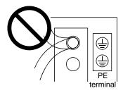
(c) If a leakage current breaker is used to prevent an electric shock, the protective earth (PE) terminals of the driver must be connected to the corresponding earth terminals.
