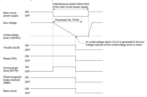
(3) When the instantaneous main circuit power failure time is longer than the set value of parameter No. PC28 (detailed setting of instantaneous power failure tough drive)
