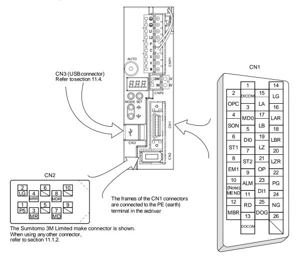
Note. Set "  $\square$  24 " in parameter No. PD16 to assign travel completion (MEND).
