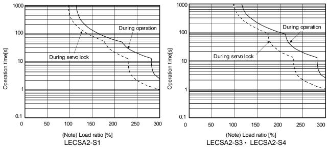
Note. If operation that generates torque equal to or higher than the rating is performed with an abnormally high frequency under servo motor stop status (servo lock status) or in low-speed operation at 30r/min or less, the driver may malfunction even when the servo system is used within the electric thermal protection area.
