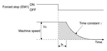
Fig. 10.3 Dynamic brake operation diagram
