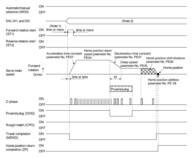
Note 1. External input signal detection delays by the input filter setting time of parameter No. PD19. Additionally, make up a sequence that changes DI0, DI1 and DI2 ahead of time by considering delays in output signal sequence from the PC or PLC...etc and variations of a signal change due to hardware.
