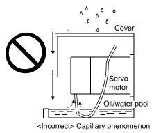
(2) If the servo motor is exposed to oil such as coolant, the sealant, packing, cable and others may be affected depending on the oil type.
