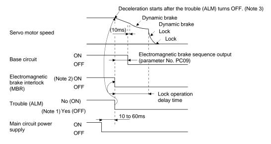
Note 1. When the main circuit power supply is off in a servo motor stop status, the main circuit off warning (E9.1) occurs and the trouble (ALM) does not turn off.
