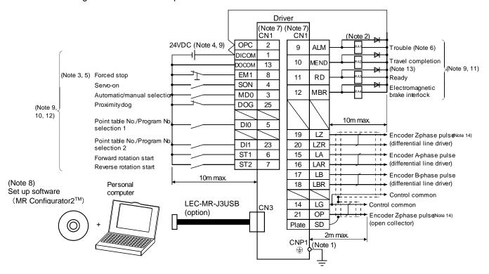
When connecting the CN1-23 pin and CN1-25 pin, supply the + 24V to OPC.
