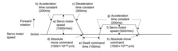
Use of an S-pattern acceleration/deceleration time constant allows sudden operation to be eased at the time of acceleration/deceleration. When the "STD" command is used, parameter No. PC03 (S-pattern acceleration/deceleration time constant) is ignored.
