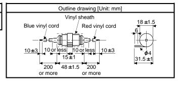
Note that a diode should be installed to a DC relay, DC valve or the like.
