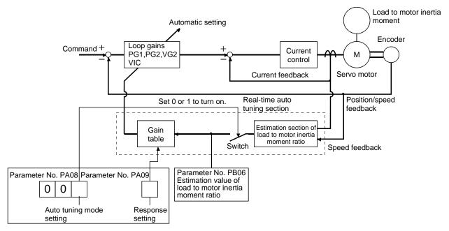
When a servo motor is accelerated/decelerated, the load to motor inertia moment ratio estimation section always estimates the load to motor inertia moment ratio from the current and the speed of the servo motor. The results of estimation are written to parameter No. PB06 (load to motor inertia moment ratio). These results can be confirmed on the status display screen of the software(MR Configurator2<sup>TM</sup>) section.
