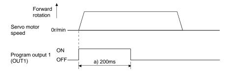
When the "TRIP" and "TRIPI" commands are used to set the position addresses where the "OUTON" and "OUTOF" commands will be executed.
