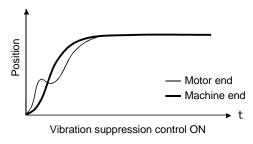
When the advanced vibration suppression control (vibration suppression control tuning mode (parameter No. PB02)) is executed, the vibration frequency at machine end can be automatically estimated to suppress machine end vibration.
