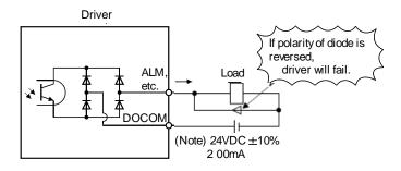
Note. If the voltage drop (maximum of 2.6V) interferes with the relay operation, apply high voltage (up to 26.4V) from external source.
