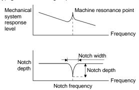
The vibration of three resonance frequency can be suppressed by the machine resonance suppression filter 1, machine resonance suppression filter 2 and machine resonance suppression filter 3.
