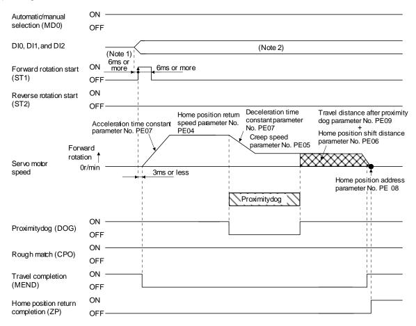
Note 1. External input signal detection delays by the input filter setting time of parameter No. PD19. Additionally, make up a sequence that changes DI0, DI1 and DI2 ahead of time by considering delays in output signal sequence from the PC or PLC...etc and variations of a signal change due to hardware.
