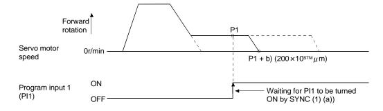
If the travel distance of the "ITP" command is less than the travel distance necessary for deceleration, the actual deceleration time constant becomes less than the set value of the "STB" command.
