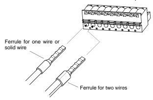
Use a ferrule for two wires when inserting two wires into one hole.
