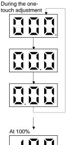
The progress of the one-touch tuning is displayed from 0 to 100%. During the one-touch tuning, the decimal point is lit, moving from right to left. Pressing the "MODE" button during the one-touch tuning calls the status display.
