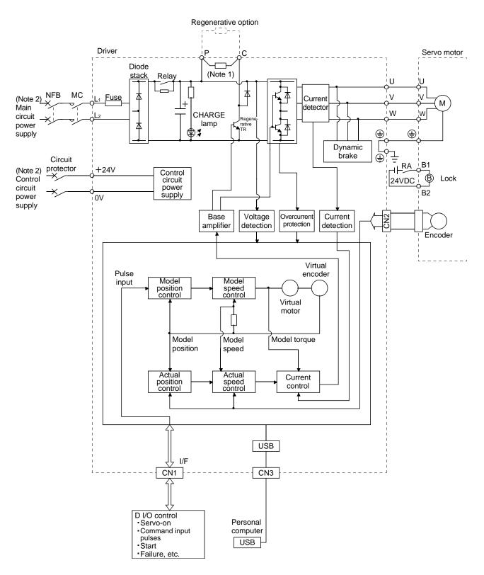
Note 1. The built-in regenerative resistor is not provided for LECSA  $\square$  -S1
