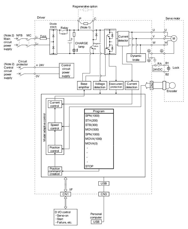
Note 1. A built-in regenerative resistor is not provided for the LECSA□-S1.
