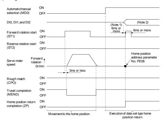
Note 1. External input signal detection delays by the input filter setting time of parameter No. PD19. Additionally, make up a sequence that changes DI0, DI1 and DI2 ahead of time by considering delays in output signal sequence from the PC or PLC...etc and variations of a signal change due to hardware.
