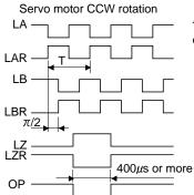
Time cycle (T) is determined by the settings of parameter No.PA15 and PC13.
