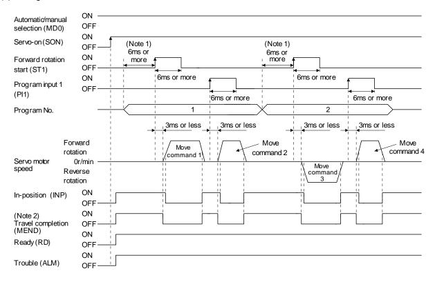
Note 1. External input signal detection delays by the input filter setting time of parameter No. PD19. Additionally, make up a sequence that changes the program selection ahead of time by considering delays in output signal sequence from the PC or PLC...etc and variations of a signal change due to hardware.
