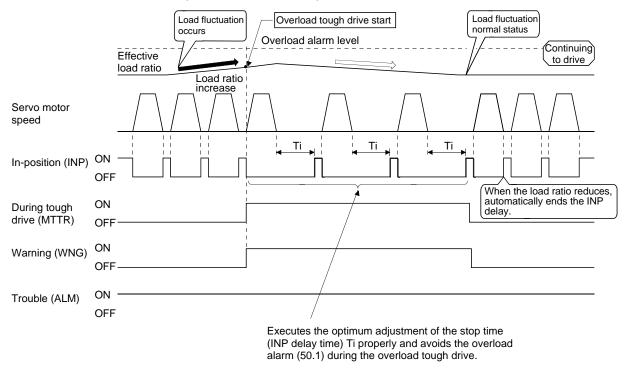
When the overload tough drive function activates, the number of tough drive in the display mode (alarm mode) is increased by one. (Refer to section 5.5.)
