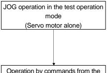
(a) Confirm that the driver and servo motor operate properly. With the servo motor disconnected from the machine, use the test operation mode (JOG operation) at the slowest speed and check whether the servo motor rotates correctly.
