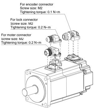
(3) The servo motor fitting part of each connector is provided with a splash-proof seal (O ring). When installing the connector, take care to prevent the seal (O ring) from dropping and being pinched. If the seal (O ring) has dropped or is pinched, a splash-proof effect is not produced.
