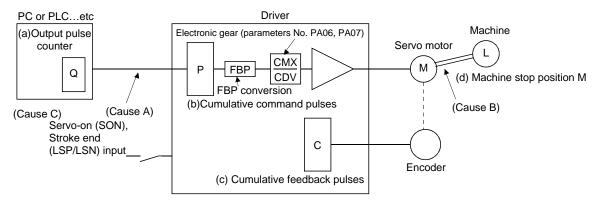
When a position shift occurs, check (a) output pulse counter, (b) cumulative command pulse display, (c) cumulative feedback pulse display, and (d) machine stop position in the above diagram.
