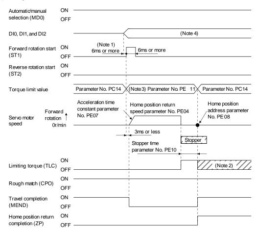
Note 1. External input signal detection delays by the input filter setting time of parameter No. PD19. Additionally, make up a sequence that changes DI0, DI1 and DI2 ahead of time by considering delays in output signal sequence from the PC or PLC...etc and variations of a signal change due to hardware.
