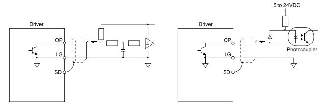
If the encoder Z-phase pulse is open collector method, it supports only to the sink (NPN) type interface. It does not correspond to the source (PNP) type interface.
