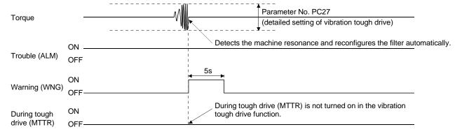
When the vibration tough drive function activates, the number of tough drive in the display mode (alarm mode) is increased by one. (Refer to section 5.5.)
