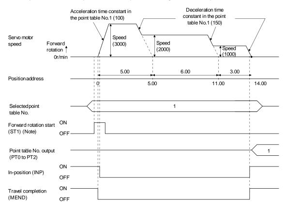
Note. Turning on reverse rotation start (ST2) starts positioning in the reverse rotation direction.
