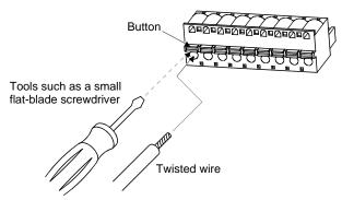
(b) Putting the wires together using a ferrule Insert the wire as the uneven side of the crimped ferrule collar faces the button side.
