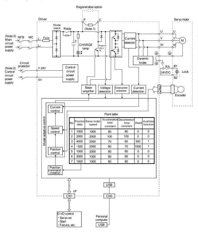
Note 1. A built-in regenerative resistor is not provided for the LECSA□-S1.
