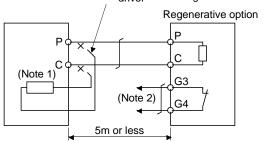
Note 1. A built-in regenerative resistor is not provided for the LECSA□-S1
