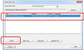
Fig.4.3 Installation of GSDML file
