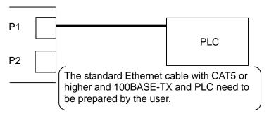
\* Cable can be connected to either P1 or P2. Follow the topology of PROFINET communication for details.
