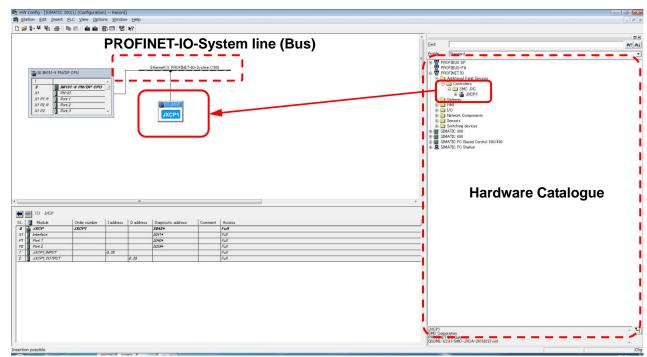
Fig. 4.4 Addition of JXCP1 to PROFINET network
