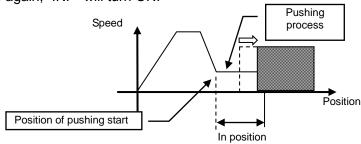
[2] Movement of the workpiece in the direction opposite to the pushing direction (The actuator is pushed back since the reaction force from the workpiece is too large.)
