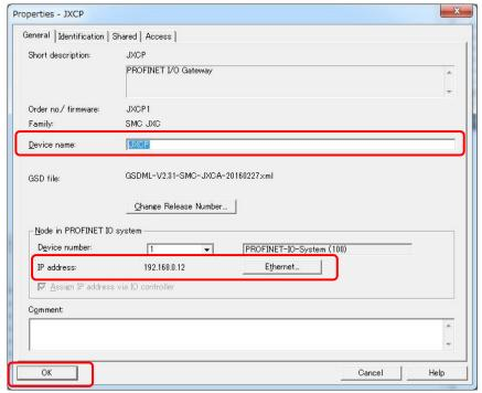
Fig.4.5 Device name and IP address input screen
