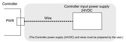
\* Refer to 6. CN1: Power supply plug (P.23) for wiring.
