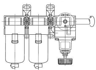
(2) Do not apply torsion or bending moment other than the weight of the product itself. The external piping should be supported separately because it may cause breakage.
