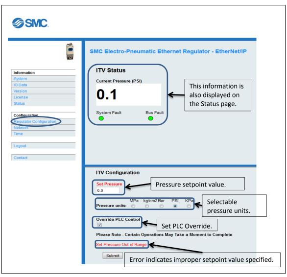
Figure 35 - ITV Regulator Configuration Page
