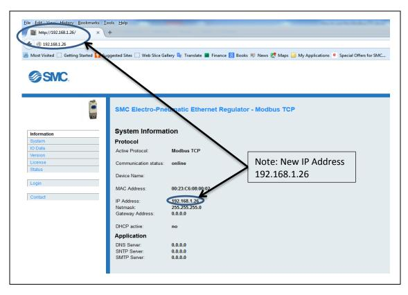
Figure 21 - New ITV IP Address In Effect
