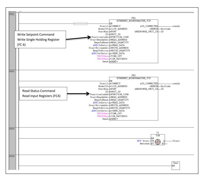
Figure 42 - Example Wago PLC Function Block Ladder Logic
