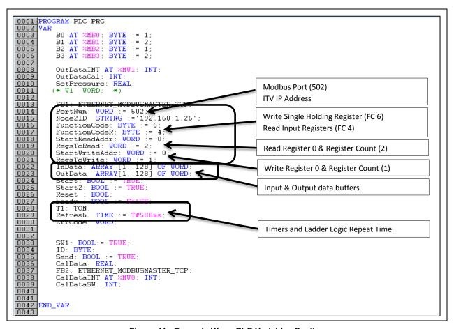
Figure 41 - Example Wago PLC Variables Section
