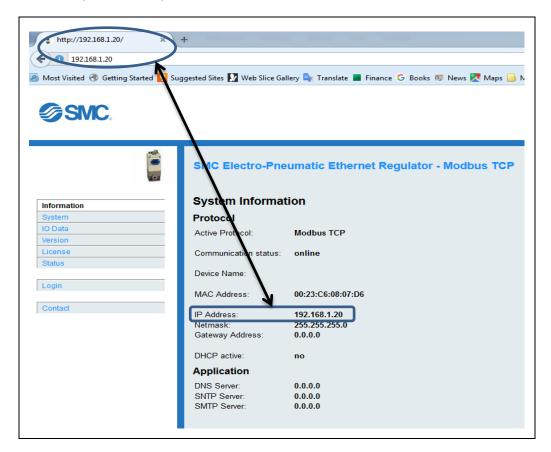
Figure 18 - ITV "System Information" Page with Factory Default IP Address
