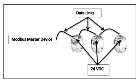
Figure 11 - Example (non-POE) ITV Data and Power Connections
