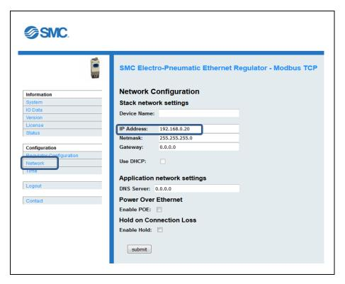
Figure 20 - Network Configuration Page Loaded
