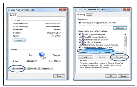
Figure 15 - Windows Local Area Connection and Local Area Connection Properties
