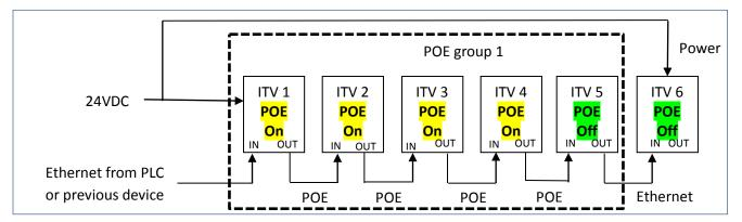
Figure 23 - ITV POE Group Ethernet Connections
