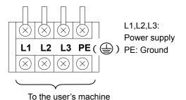
Terminal connecting screw: M4 Crimped terminal width: 9.5mm or less Applicable electric wire: 5.5mm<sup>2</sup> or more
