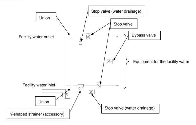
This equipment and facility water piping should be easy to disassemble so that the water-cooled condenser can be cleaned.
