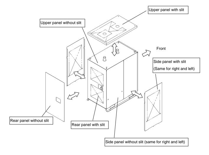
Replace the panel to which ventilation should be directed with one with slit, and the panel where ventilation was previously directed with a panel without slit. For ventilation to the top, be sure to use the product indoors.
