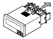
Lift up the end of the battery and remove.
