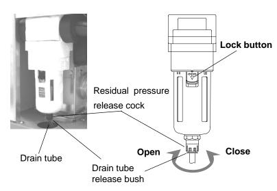
pen the residual pressure release cock at the drain tube connection port to release air and drain fluid left in the product.
