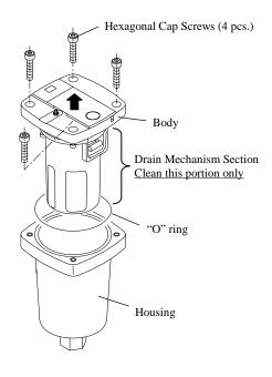
Figure 2: Disassembling Diagram
