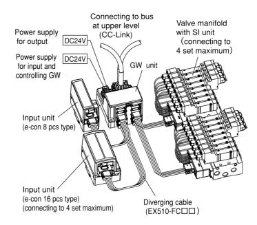
System in which realize wiring saving and distributed installation by connecting to Fieldbus. Signal to Fieldbus is transmitted by GW unit, and signal to input/output device which is installed distributed is collected by GW unit.
