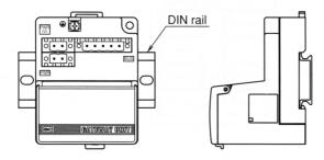
Put Claw 1 at the body under DIN rail and push it upward. Push down Claw 2 to the opposite rail until the claw clicked to be set stably.
