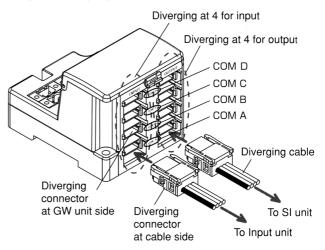
Insert branching connector on the table side from the bottom (COM A, B, C, D of branching connector of GW unit side).
