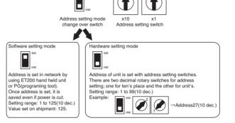
\*: When software setting mode is selected, address setting switches are not effectual. Moreover software setting mode and hardware setting mode differ in ID numbers of units.
