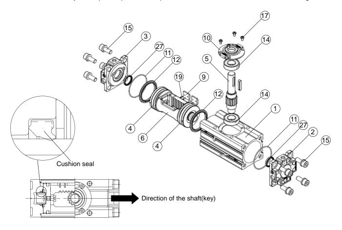
Fig. (18) Direction of assembly of the shaft
