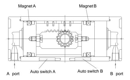
Fig. (16) Auto switch operation principle
