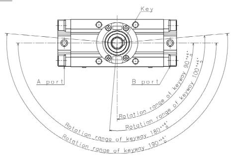
Fig. (2) Rotation range of shaft keyway (size 50 to 100)
