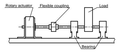
Fig. (9) Flexible coupling
