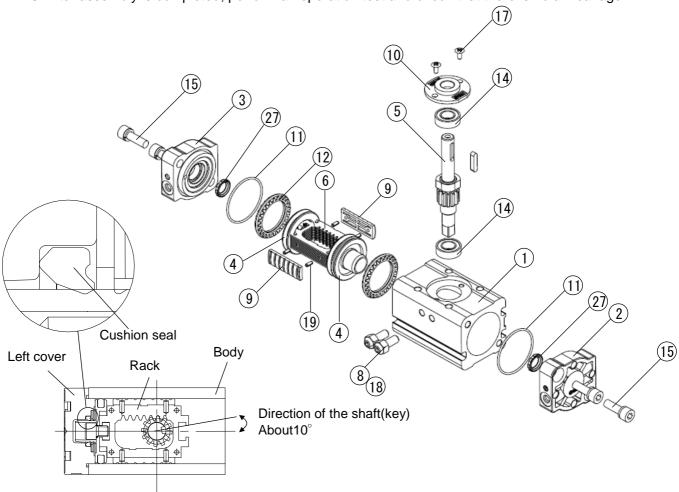
Fig. (17) Direction of assembly of the shaft
