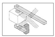
The external stopper be- If an external stopper is incomes a fulcrum, resulting stalled on the shaft side in the load's inertia force which is opposite of the being applied to the shaft load, the inertia force generated by the load is applied directly to the shaft.
