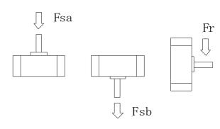
Point of application of force of Fr is the center of shaft flat face and longer dimension of the key.
