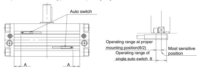
Fig. (14) Proper auto switch mounting position
