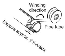
Fig. (11) Wrapping of pipe tape
