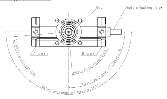
Fig. (3) Rotation range of shaft keyway (angle adjustable type)
