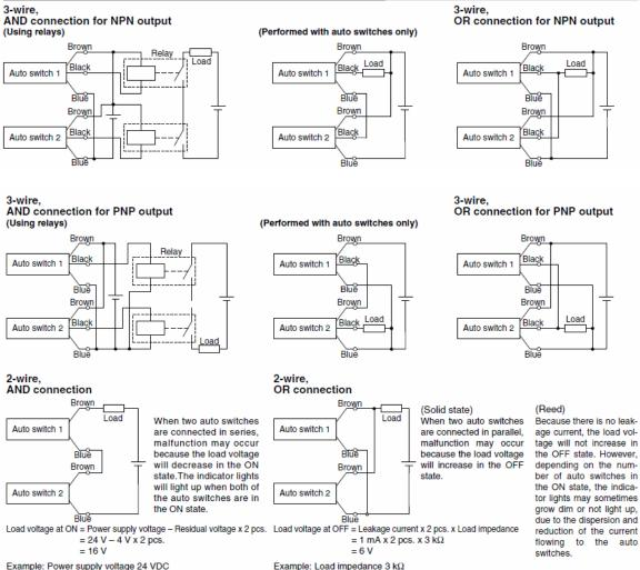
Example: Power supply voltage 24 VDC Auto switch internal voltage drop 4 V
