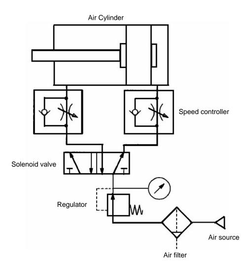
Fig.3 Basic Circuit
