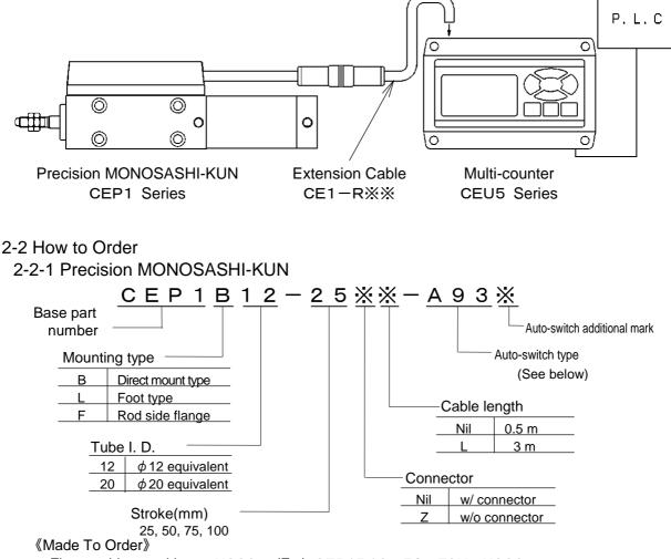
Fluoro rubber packing: -XC22 (Ex.) CEP1B12-50-F9N-XC22
