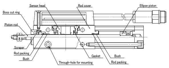
• A part of the piston rod has scale (magnetic scale). In order to maintain the relative position of the scale and the sensor head, ellipse piston is used to have a structure of non-rotating cylinder.
