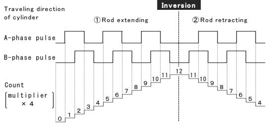
①In rod extending direction, A-phase turns on first, then B-phase turns on with the delay of approximately 90° phase difference.
